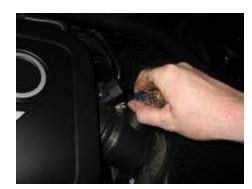
Using your Phillips head screwdriver loosen the hose clamp next to the MAF housing.
