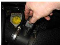
Firmly grasp the plug on top of your MAF sensor unplugging it. Lay the plug back away from the intake system.
