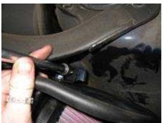
Next, line up the "L" shaped bracket on the side of the air box, using the same bolt that secured the factory air box. Tighten that bolt through the bracket into the same hole that it originally used. This will secure the V-Flow to the car.
