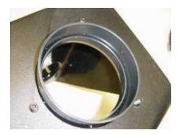
Locate the V-Flow air box. Notice one side has a large hole with three smaller holes equal distance apart surrounding the large circular hole. Picture the air box as a complete box and place the 6" ventrui inside the box. Turn the orientation of the venturi so that the lip of the ventrui and the 3 threaded studs poke through the box to the outside of your air box.
