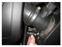
You will notice a hose with a 90 degree bend and a small plastic ring around the end of it snapped into place at the bottom of the factory air box. Firmly squeeze the top and the bottom of that ring squeezing together and pull the hose off of the factory air box. Pull the hose back and tuck it back out of the work space.
