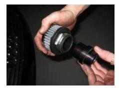
In your kit there is a small anodized black billet aluminum adaptor. One end is round, and the other end has two notches cut out of it. Slide the small breather filter over the round end of your adaptor and tighten the hose clamp.
