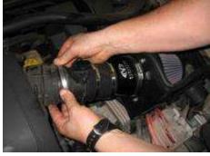
Insert your V-Flow unit into the space that the factory air box used to be. Make sure the MAF is pointing in the direction of the engine and the filter is pointing in the direction of the fender. Slide the turbo inlet hose over the open end of the MAF housing and re-use the same hose clamp that you originally loosened during the removal of the factory air intake system.
