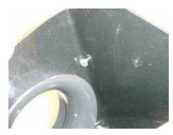
On the inside corner of the air box you will notice a small hole. Take the 11mm bolt that is included in the kit, from the inside of the air box slide the threaded end through to the outside. You may need to use some force to slide it through the plastic.
