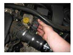
Take the wiring harness that was originally plugged into your MAF sensor and plug your MAF sensor back in
