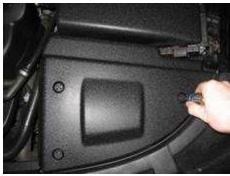
Start with your Phillips head screw driver and remove the three screws on top of your battery cover. Then remove the battery cover from the car.
