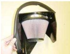
Loocate the section of weather stripping take notice there are two small sections that are cut out of one side of the weather stripping. Those cut outs are to allow the weather stripping to bend around the corners of the air box. Because of those cut outs there is only one way that the weather stripping can be installed. After you determine the orientation of the weather stripping, push it onto the top of the air box.
