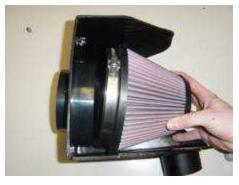
Take the 6" filter and slide it onto the venture. Be sure to keep the hose clamp facing up so that you can tighten the clamp around the filter.
