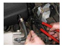
Take the wire clippers and clip off the end of the zip tie to remove the unneeded slack.
