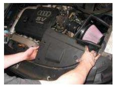
Using the Phillips head screwdriver, re-attach the factory battery cover to secure it, using the three Phillips head screws. After you replace these screws, your new V-Flow is installed and ready to go. Make sure all hose clamps are tightened and all tools are removed from your engine bay and enjoy your new intake.
