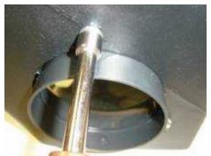
Take three of the four 11mm nuts that are included in your kit and thread each of the three nuts onto the three studs that are attached to the venturi. Tighten them down against the air box using your 11mm socket or nut driver.
