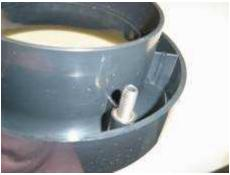
Next, take your 6" venturi and your 3 threaded studs. The studs will have one end with red on it. This red end is threadlock, insert the red end into the venturi and tighten each stud using the 3mm alen wrench. Tighten them until the red section is completely inserted into the holes in the venturi.
