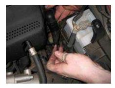
If you follow the smog pump hose down a few inches from the 90 degree bend you will find another similar looking ribbed style plastic hose. Line up the smog pump hose along side the second ribbed style plastic hose. Then take the black zip tie provided and wrap it around both hoses pulling it tight, as shown here. This will keep the breather filter from moving around unprotected.
