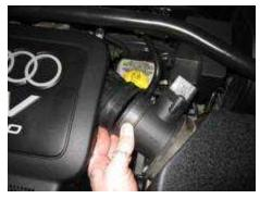
Grasp the hose connecting to the MAF housing and remove it from the MAF housing. Let it rest up against the MAF housing
