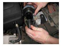
The smog pump hose, (small diameter ribbed plastic hose) that was originally attached to the side of your factory air box has, at the end of it, a 90 degree bend. Grasp the hose firmly and twist the 90 degree end about 20-30 degrees in the direction of the engine. Then, take the small breather filter attached to the aluminum adapter and attach the end of the smog pump hose to the end of the aluminum adapter. If you line up the hose just right it should snap right into place.
