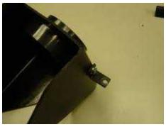
After you slide the 11mm bolt through the air box, place the small "L" shaped bracket on the bolt and then tighten the last remaining 11mm nut onto the end of that bolt. Make sure that the bottom of the "L" shaped bracket is down, parallel with the bottom of the air box as shown in the picture.
