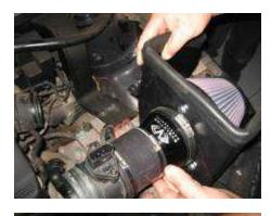
Next, take the MAF with the attached silicone coupler that you assembled earlier, and attach the other end to the adapter.
