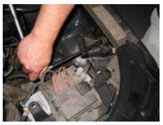
If your car has this fresh air duct, take your 10mm socket, remove the nut that secures the factory fresh air duct to the side of the fender. Then remove the short piece of ducting.
