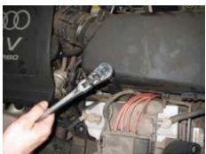
Take the 10mm socket, extension, and wrench. Remove the two bolts that secure the factory air box to the car. One is behind the negative battery terminal and the other is at the opposite corner of the air box, in front of the driver's side strut tower.
