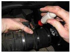
Twist the MAF housing so it is pointing in the same direction that it was when it was installed on the factory air box. Tighten down the remaining hose clamps that may be loose.
