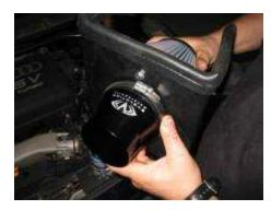
Take the 3-9/16 - 4-/12 size hose clamp and slide it onto the small lip on the outside of the venture. Then take your \*MAF adapter and slide it into the outside of the venturi, tightening the hose clamp.
