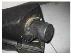
Attached to your air box, which has now been removed from your car, is the housing for your MAF sensor.
