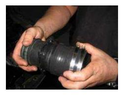
Next, take the silicone reducer and slide the smaller end onto the MAF housing. If you look at your MAF housing you will notice an arrow indicating air flow. Make sure that arrow is pointed away from the silicone reducer. Another way to be sure you are attaching the silicone reducer to the proper side, is to note that the reducer goes on the same side that used to be on the outside of the factory air box when the MAF housing was attached to it.
