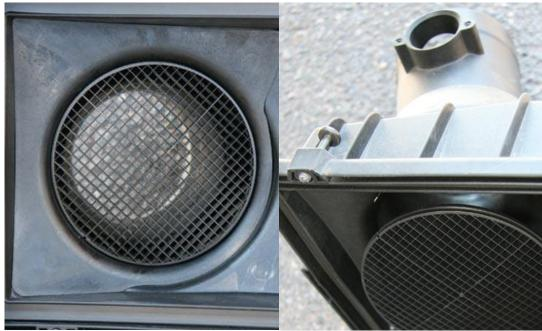
2. Install the OEM MAF waffle into the EVO billet Venturi. It will snap into place like it did in the OEM airbox. NOTE: the waffle is concaved and is directional. The concaved section of the waffle is the back side. Install the waffle in the same direction that it was installed in the OEM airbox.
