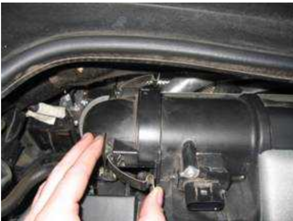
You will find two silver clamps that attach the turbo inlet hose to the MAF. Remove clamps on both sides of that hose.
