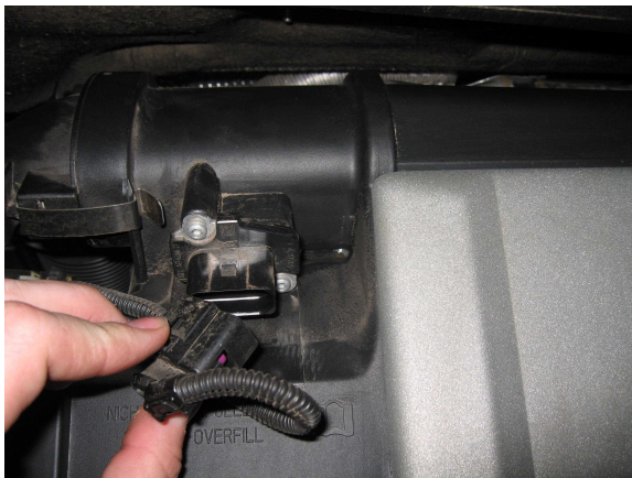
Start by unplugging the MAF sensor at the top of the engine cover.
