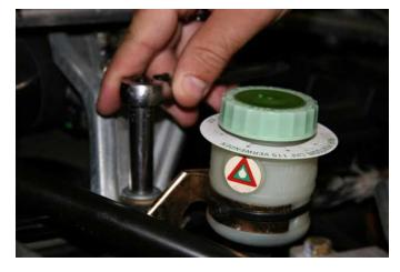
Remove the 10mm bolt that connects the hydraulic reservoir bracket to the car
