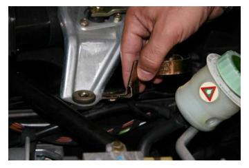
Remove the hydraulic reservoir bracket
