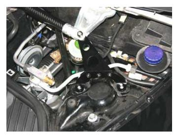
Fit one side of the strut brace onto the OEM strut studs. Please make sure that the billet bracket is fully seated on the strut tower before moving to the next step.
