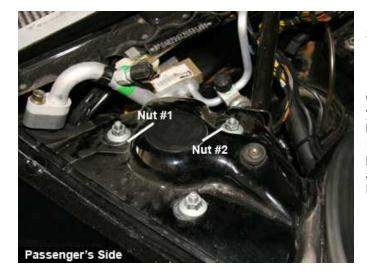
Once the battery covers are removed, you will see that there are three 13mm bolts located on the strut tower. Remove the two bolts labeled in the picture to the left. Put these bolts aside because you will reuse them later on in the installation.
