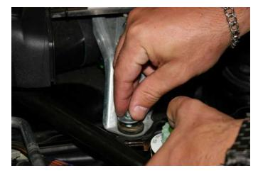
Re-attach the 10mm bolt that holds the hydraulic reservoir bracket to the car.
