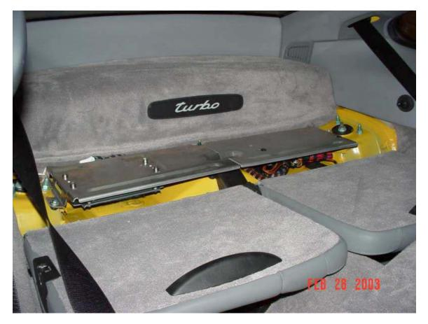
There are two 10mm bolts and a 10mm nut. As located in the pictures remove these fasteners on the left side only.
