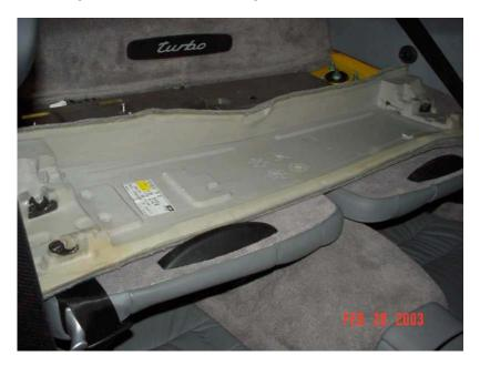
Remove the lower carpet section. (on the Bose Sub cars there is three pieces of carpet, only two need to be removed.) You can see from the pictures the carpet is foam backed and is not held in with anything other than pressure. Simply pull from he front or back and remove the lower carpet.
