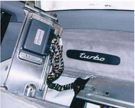
Flip the metal panel up and remove the 4 10mm nuts from the ECU.
