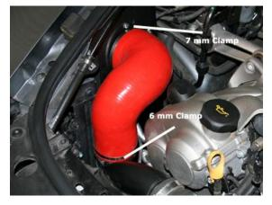
12) Secure the top of the supplied V-Flow red silicone intake tube to the venturi using a 7 mm ratchet. Secure the bottom of the red silicone hose to the MAF housing a 6 mm ratchet.
