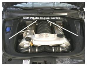
1) Using a flat head screw driver, remove the plastic OEM engine covers by unscrewing the large plastic hold down clips. These only require a 1/4 turn to remove.
