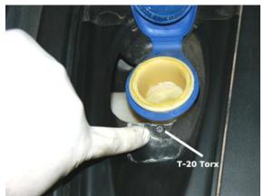
2) NOTE: The passenger's side engine cover also has a T-20 Torx that must be removed
