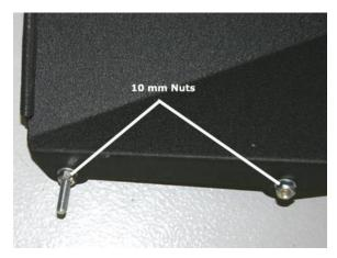
8) Tighten the supplied 10 mm nuts and bolts to the bottom of the EVO heat shield. NOTE: Make sure that there is a washer on both sides of the 10 mm nut.
