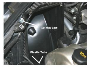
7) Remove OEM air box cover and filter. This will pull out at this point exposing the air box back housing as shown in this photo.
