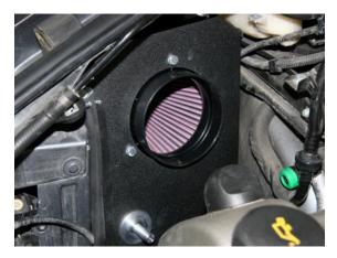
11) Place the V-Flow heat shield assembly into the engine compartment.
