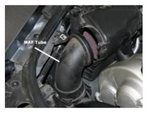
5) Using a 7mm ratchet, loosen the hose clamp that secures the MAF tube to the turbo inlet tube. This clamp is not shown in this photo and it is located on the downward side of the MAF housing.
