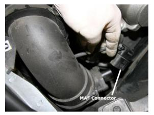
3) Unclip the MAF (Mass Air Flow Meter) connector.
