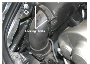
4) Remove the OEM air box cover by rotating the two locking bolts 180 degrees and then pulling them straight up. You will need to do this with a pair of pliers.
