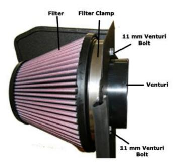
9) Attach the supplied Venturi to the heat shield with the supplied 11 mm bolts.
