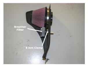
10) Insert the supplied billet aluminum air ride breather filter adapter through the heat shield as shown.
