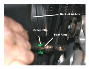
6) Remove the air ride connection that is located on the back of the air box assembly. First pop off the green vent clip with a small flat head screwdriver or pick. Next, push the seal ring away from the air box with a flathead screwdriver as shown in the photo to disconnect the air ride vent line.
