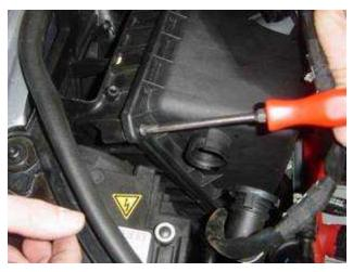
For easiest removal, the airbox must be separated into two pieces to be removed from the car. Loosen all the screws holding the top of the airbox to the bottom half.
