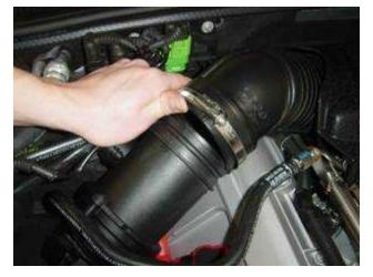
Loosen the hose clamp on the rubber hose connecting to the MAF housing. Remove screws holding MAF housing to airbox to await new tube installation. This will allow for easy adjustments when fitting the intake tube.
