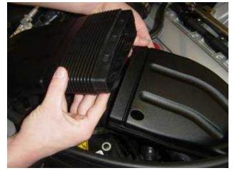
Remove the fresh air ducting that feeds into the factory airbox from the front grill. The ducting separates into two parts manually by hand.
