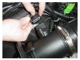
Disconnect the MAF sensor plug from the housing. Note: there is an arrow on the MAF housing that corresponds to a line on the rubber inlet hose. These must be re-aligned after installation
