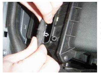
The wiring harness that attaches to the airbox is held into place by several snap in connectors. You can use a screwdriver to pry them out.
