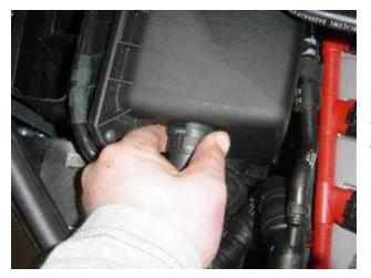
Disconnect the secondary air pump hose from the OEM airbox. Squeeze the ends of the ring around the clip and pull.
