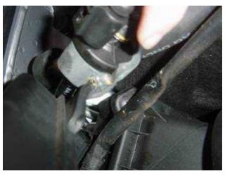
Remove the purge canister connected to the airbox, the entire rubber grommet holding the canister into place slides off the plastic arm.
