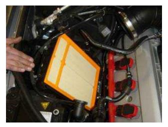
The top section will easily disconnect from the bottom assembly once screws have been removed, you can now remove the filter
