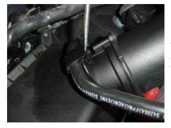
On the top of the box near the MAF housing is a snap clip that secures a fuel line. This clip opens towards the front corner of the car to free the line.
