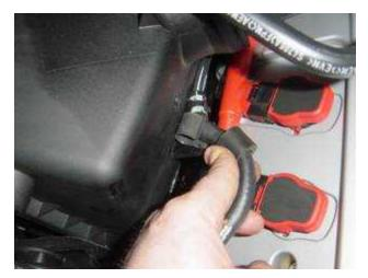
There is a line that runs along the airbox. It is held into place by a metal spring clip. The hose simply pulls out of the clip.
