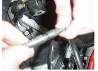
There is a vacuum line that connects to the back corner of the airbox (back corner of passenger side). If you follow this line there is a 2-way connector a few inches outside the box that can be disconnected.
