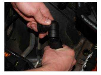
Remove the 90-degree secondary air line connector.
