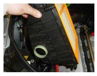
The bottom half of the airbox can now be removed from the car. There is a fresh air duct at the bottom that can be disconnected by slightly pulling the box towards the rear of the car, then upwards. The box is held in by rubber grommets so may require a little force.
