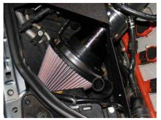
Install the EVO V-Flow air filter to the EVO plastic venturi, which is attached to the billet aluminum Venturi tube. Install this entire assembly as shown with the silicone hose and hose clamps. Make sure all hose clamps are tightened, and the MAF housing is aligned in its original position.
