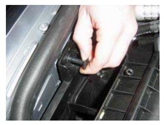
The airbox is connected to the fender by an expanding clip. To remove the clip you can pull out the center pin and it will release from the fender.
