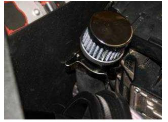
Install the supplied breather filter into the secondary air hose and secure to the spring clip already fastened to the heat shield.
