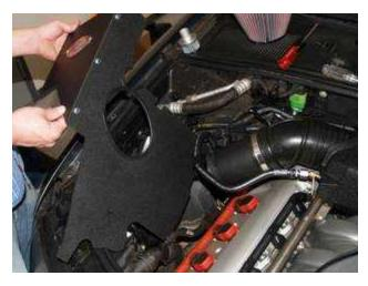
Install the EVOMS V-Flow heat shield in the car. The top cover attaches to the heat shield by 3x 10mm bolts with 3x small washers. This step and the next should be done simultaneously for easier fitment purposes.
