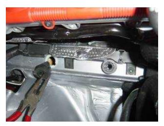
Remove the rubber grommets from the frame rail to prepare installation of the V-Flow heat shield.
