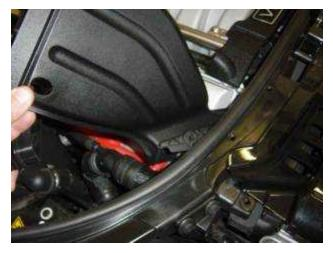
The portion of the duct that attaches to the front grill is held into place by two Phillips screws. Remove these and complete the disassembly of the fresh air ducting.
