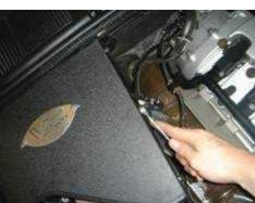
Now, take your 10mm wrench, or socket and finish tightening the three 10mm bolts that you finger tightened earlier in this install. This should close the gap in between the two sections of the heat shield and give it a nice clean look.
