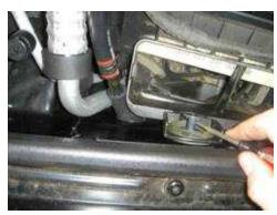
On the inside of the drivers fender there is a small plastic plug inside a rubber grommet, located above the air box. Take your flat head screw driver, and work the plastic plug out. This should be the last thing securing the factory air box in place.
