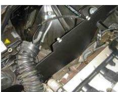
The vertical section of your heat shield should look like this after install; With the Nutserts and the tab holding the 13mm nuts pointing to the passenger side of the car.
