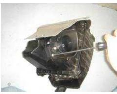
Using your Phillips head screw driver remove the two Phillips head screws out of the MAF housing and remove the whole unit from the air box.
