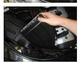
First remove the front section of the fresh air inlet
