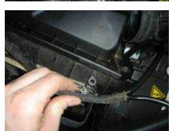
There are some wires, including the wires running to your MAF plug. They are held into the air box by small push in clips. Gently work those clips out and pull the wires aside, out of the way.
