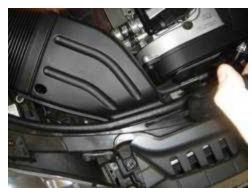
Start with your Phillips head screw driver and remove the two screws that attach the factory fresh air inlet at the core support.
