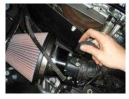
Plug the MAF plug back into the MAF sensor.
