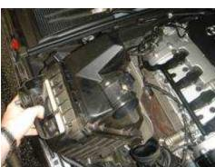
Firmly grasp the factor air box. As you pull straight up it should un-snap from two rubber grommets underneath. If the rubber grommet stays attached to the air box remove it from the air box and push it back into its spot in the engine bay.
