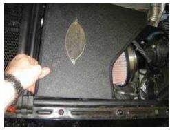
Grab the horizontal section of the heat shield and tuck it under the edge of the fender. That is why the holes are slightly misaligned, so that there is enough tension to keep the heat shield firmly up against the fender.
