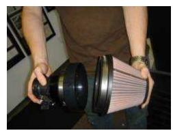
Take the Venturi, adapter and MAF section that you just assembled and attach it to the filter that we provided for you. Then tighten the hose clamp around the base of the filter.
