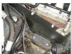
Attach the two 13mm bolts with nuts to the vertical section of your heat shield (the larger section without the V-Flow logo) Make sure the long end is pointing down, away from the heat shield. Work the heat shield into place with the bolts pointing down, and the bent tab pointing to the passenger side of the car.
