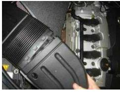
Then take the front section of the factory fresh air duct, line up the holes in their original place in the core support and then attach the two sections in the middle as shown here.
