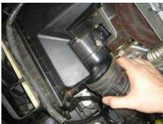
**Remove turbo inlet hose from the MAF** housing attached to the air box, and pull it back out of the way, tucking It under the core support.
