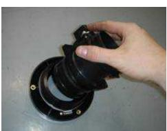
After you have your MAF housing positioned in the right direction place the end of it into your Venturi. You will probably have to use some force to fit it in, but push down firmly until the MAF housing slides into the Venturi adapter.
