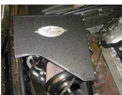
Take the 10mm bolts, with washers and slide them through the holes in the horizontal section of your heat shield and finger tighten them into the vertical section. Again, it will seem as though the holes don't line up. Your horizontal section of your heat shield should be angled up slightly.
