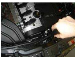
Replace both screws into the core support fastening the factory fresh air duct back into place.
