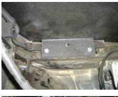
Line up the two bolts with the two rubber grommets that are still attached to the car. Push the bolts into the grommets letting the heat shield rest inside them.
