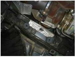
The two rubber grommets that your factory air box snapped rested in are pictured here. This is where you will also attach the vertical part of your heat shield.
