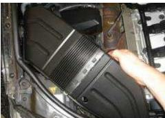
The factory fresh air inlet is put together in two pieces, separate them in the middle
