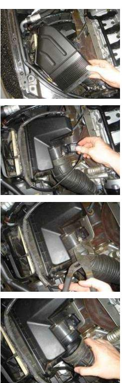
Then remove the rear section of the fresh air inlet
