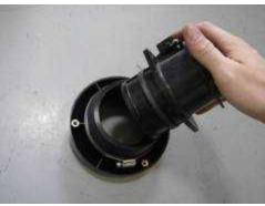
Place your Venturi on a hard flat surface face down. Take your MAF housing; locate the arrow on the side. Position the MAF so that the arrow indicating air flow is pointing away from the Venturi.
