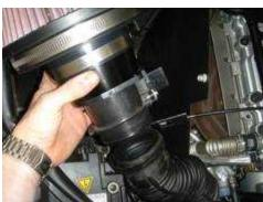
Place the filter, Venturi, adapter, and MAF unit into the end of the turbo inlet hose. Be sure to point the MAF sensor in the same orientation that it was originally pointed when it was sitting inside the factory air box before you removed it. Then place the hose clamp back on the end of the turbo inlet hose.
