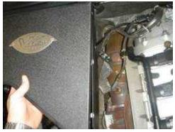
Take the horizontal section of your heat shield, the smaller piece, (the one with the V-Flow logo) position the holes in that section to line up with the Nutserts in the vertical section of the heat shield. It will seem as though it doesn't line up perfectly but that is ok.
