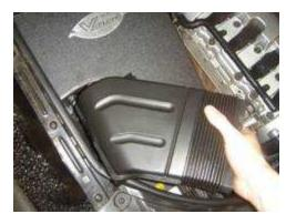
Now, take your original factory fresh air duct. Placing first the rear section tucking it down in between the heat shield and the core support.
