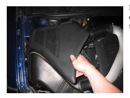
Remove black air box cover on left side of engine compartment. The cover is held in place with three spring clips located in a triangular pattern.
