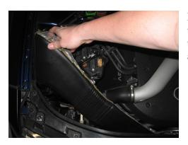
Remove fresh air feed tube by pulling the left side off the OEM air box first. Then unscrew the two screws at the core support and pull off the front side if the fresh air feed.
