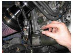
On your heat shileld you will notice a tab bent in the direction of the motor, slide the other black metal clip onto that tab.
