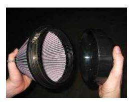
Take the filter and 6" ventrui, slide the rounded edge of the venturi inside the filter and tighten the hose clamp.
