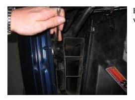
Remove the 10 mm nut from passenger side fender wall. Also remove the two washers.
