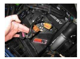
Unplug the four ignition igniter plugs on the OEM air box and note the placement. Move the harness and plug ends to side by detaching them from the in air box fasteners. Also detach and move rubber fuel lines off to side. Note: There is an additional wire clip located on the front bottom side of the air box.
