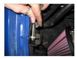
Take the small aluminum tab and attach it to the side of the fender, utilizing the same 10mm bolt that the OEM air box mounted too. Then take one of those black metal clips that you removed from the top of your OEM air box in the previous step, and clip it onto the top of that aluminum tab.
