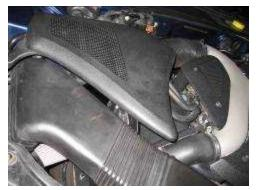
Replace the OEM air box cover by clipping one side into the aluminum tab on the fender, and the other side into the tab of the heat shield. This will help hold the heat shield up away from the motor.
