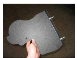
Put supplied M8 hex head cap screws through the bottom of the heat shield and tighten the M8, nylon-insert locknuts on the underside. Tighten firmly with a 13mm socket and wrench.
