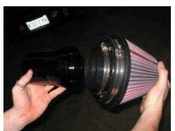
Get the intake tube ready for installation. Make sure the inside of the new intake tube is free from debris. With tube held vertically, place the large end inside the venturi/flter unit.
