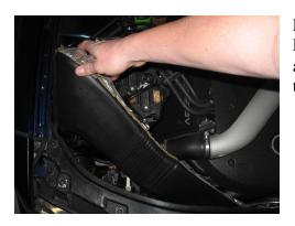
Replace the OEM fresh air duct into its original place, letting the open end point downward on top of the filter and sliding the other end into the core support lining up the holes for the two phillips head screws.
