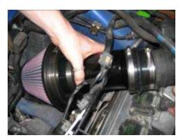
Slide the intake tube, filter, and venturi that you previously assembled into the open end of the coupler, keep the wires for the ignition modules on top of the tube as you slide it in.
