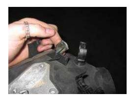
On top of your factory air box you will find three metal clips that your OEM air box cover cliped into. Remove two of those clips from on top of your air box.
