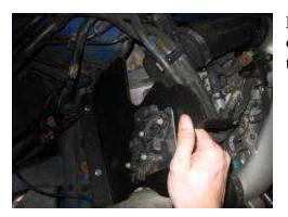
Place heat shield in car with bolts inserting into the orange grommets. The bent tab on top should point towards the passenger side.
