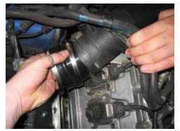
Place the coupler on the end of the MAF housing with both hose clamps. The clamp around the MAF housing can be tightned all the way. Tighten the clamp on the open end of the coupler just enough so that it doesn't fall off. But not too tightly that you cannot slide the intake tube into it.
