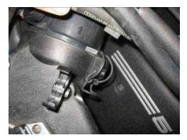
Next, unclip the lever style clips connecting the MAF sensor assembly to the OEM air box. If the black Oring comes out, place to side.
