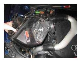
Pull the air box towards the driver's side and lift straight out. After removing the air box, remove the orange grommet from the air box and place back into position inside the engine compartment. At the same time, also place the other supplied orange grommet in the other hole.
