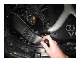
Replace the two phillips head screws into the core support and securing the factory fresh air feed.
