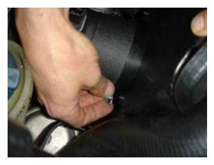
Install the included 11 mm serrated nuts on to the Venturi studs and tighten. Be sure not to over tighten, the fitment should be snug.
