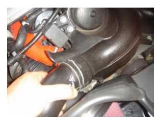
Reinstall the OEM boost hose clip. Pull on the boost hose to ensure that the hose is securely attached to Y-Pipe.
