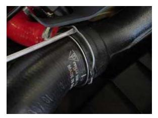
Remove clip from driver's side boost hose by slipping a flat head screwdriver in between the clip and the Y-Pipe and carefully prying the clip off.
