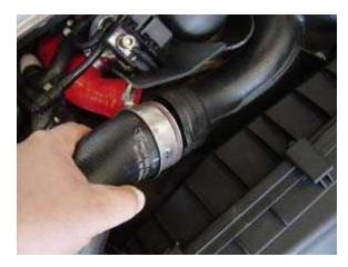
Remove the boost hose by pulling the hose out of the Y-Pipe. **NOTE:** You do not remove the hose out of the car; you simply push it to the side so that there is more room available for the install.
