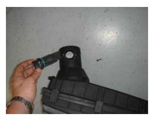
Use the included tamper proof Torx key to remove the mass air flow meter screws that secure the MAF to the OEM airbox, and remove the MAF from the stock housing.
