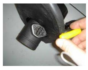
Secure the MAF to the V-Flow mass air flow/Venturi housing the supplied hardware using a 3mm Allen Key.
