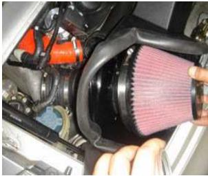
Insert the assembled V-Flow unit into the engine compartment. When inserting the V Flow air box / venturi / air filter into the engine compartment, be sure that the MAF is pointing up and the venturi studs are lined up in the area of the holes that they fit through on the airbox. Do not slide them through the holes until the entire airbox / air filter are sitting properly in the engine compartment.
