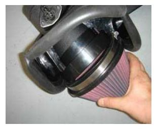
Install the supplied air filter over the injection-molded Venturi and secure it with the included hose clamp. NOTE: You will notice 2 studs that are threaded into the Venturi. Later on in the installation, these studs will be inserted into the holes that are located above the 4" opening in the airbox. It is important NOT to install the hardware and secure this to the airbox at this time. Doing so will hinder the proper installation of the unit into the engine compartment.
