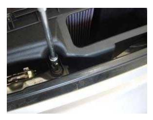
Remove the 13mm bolt located to the right of the striker plate. This bolt secures the factory air box to the body of the car. Save this bolt for reinstallation on the EVO V-Flow.
