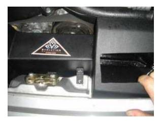
Move the airbox in place so that the airbox mounting L-bracket lines up with the OEM airbox mounting point located to the right of the decklid striker plate. Secure with the OEM 13mm bolt.
