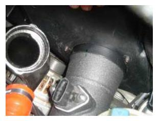
Note: Once the air box is properly seated in the engine compartment and the MAF/Venturi housing is in the proper position, the two studs that are located on the back of the Venturi housing should protrude completely through the air box.
