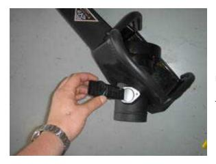
Reinstall the stock MAF into EVO V-Flow mass air flow/Venturi assembly. NOTE: Do not touch, drop, shake, or try to clean the stock mass air flow meter filament. Doing so may damage it.
