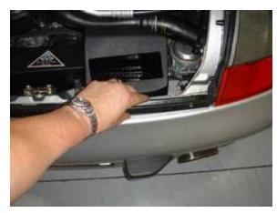
At this point, verify that all the connections have been correctly attached and or tightened, and then reinstall trim strip.
