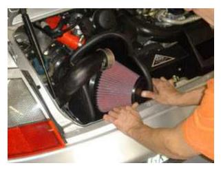
Once the airbox is in the engine compartment and seated correctly, make sure that the airbox does not sit on any of the oxygen sensor wires that are located on either side of the airbox.
