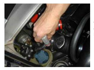
Tighten the OEM hose clamp around the OEM rubber coupler to secure the MAF housing.
