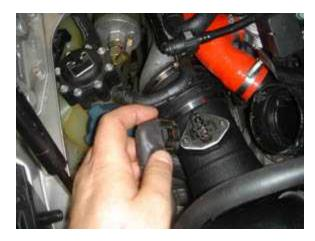
Plug in the MAF harness into the MAF meter
