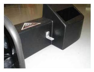
Connect the supplied L-Bracket to the V-Flow intake box using the supplied 11mm bolt. Make sure you connect short side of the L-Bracket to the V-Flow intake box, for the long side will be used to connect the V-Flow to the car. Also, make sure that the long end of the L-Bracket is facing down otherwise the box will not correctly seat in the engine compartment.
