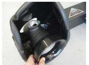
Insert MAF tube/Venturi assembly through the 4"hole in the V-Flow air box.
