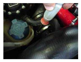
Loosen the 7mm hose clamp that attaches the stock air box to the fresh air intake plenum.
