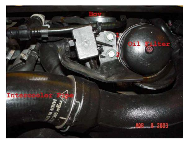
You will need to remove the clip that holds the upper hose over the BOVs. This is done by sliding the clip out as seen in the picture. Once the clip is removed you will notice the black sleeve pushes in and out of the mating portion. Pushing the hose all the way in the other section hold the inner black sleeve and pull the hose out. The metal neck will remove from the valve and will remain in the hose. Now pull the hose out of your way.
