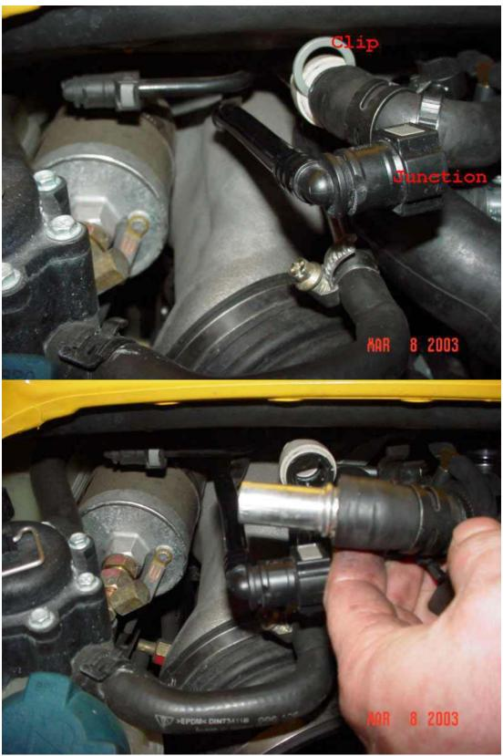
Next you will need to remove a few hoses. On hose #1 you will see a gray portion on the sides of the junction. While pressing these in pull on the opposite section of the hard plastic hose to separate. Pull the right side around and out of the way. Take caution not to bend or break this line. Next you will need to squeeze the clip of #2 together and move the hose off
