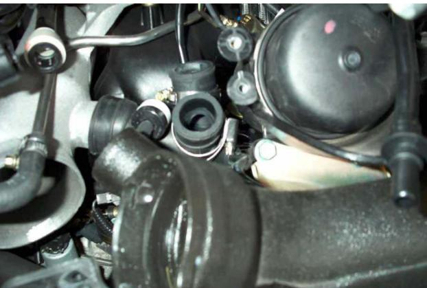
Once the three clamps from the upper BOV ports and the "Y" have been removed you can remove the connecting hose as one whole unit. Once the hose is removed you can remove the lower clamps on the BOV and pull the front BOV out. Remove the vacuum line and the lower clamp and remove the rear BOV
