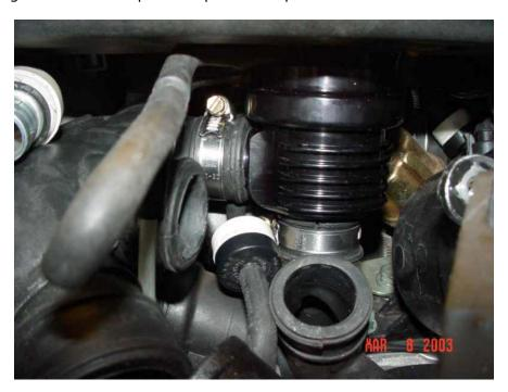
Place the connecting hose back in its spot and secure the rear side clamp. Now place the front EVO BOV in and secure the clamps and vacuum line. Re secure the main clamp back on the "Y" as removed.
