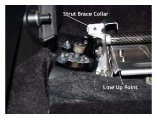
\*\*\*\*To correctly align the strut brace, try to align the strut brace collar lines to the line up point shown in the picture to the left. The end of the carbon tube should be in line with the edge of the aluminum tray.
