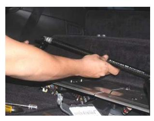
10. To adjust the bar, hold the passenger's side strut bar mounting bracket in place while twisting the carbon fiber strut bar. To move the bracket inwards, twist the carbon fiber bar clockwise. To move the bracket outwards, twist the carbon fiber bar counter-clockwise. Test fit to ensure proper length. DO NOT ATTACH STRUT BAR MOUNTING BRACKET TO THE CAR AT THIS TIME.
