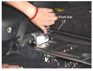
14. To re-attach the strut bar to the mounted billet bracket, push the carbon fiber bar back against the carpeting until it can slide into the mounting bracket. Once the bar is in, push the connecting bolt through the back of the mounting bracket and tighten. This process will take some force.
